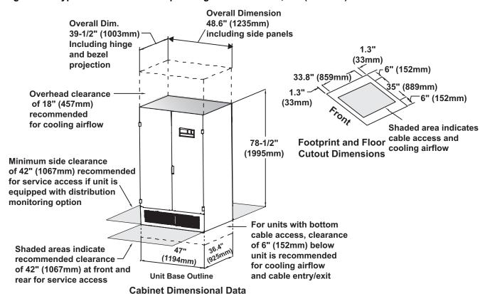
Figure 2 Typical cabinet and floor planning dimension data, 47" (1194mm) cabinet 50-300kVA
